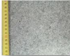
a) Sandblasted Granite Slab noted "GSSB"
