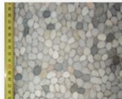
f) Rounded Sandblasted Aggregates noted "RSBA"
