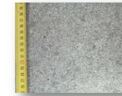
a) Sandblasted Granite Slab noted "GSSB"
