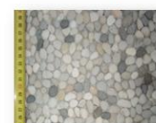
f) Rounded Sandblasted Aggregates noted "RSBA"
